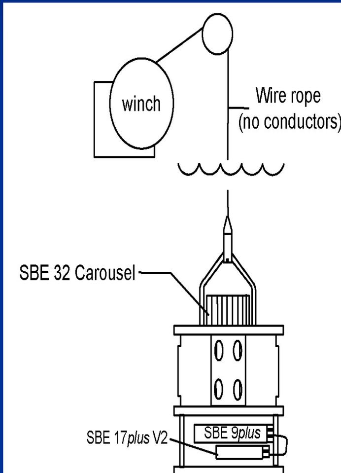
The PLASMA does not have an electrical or fibre optic core.....
